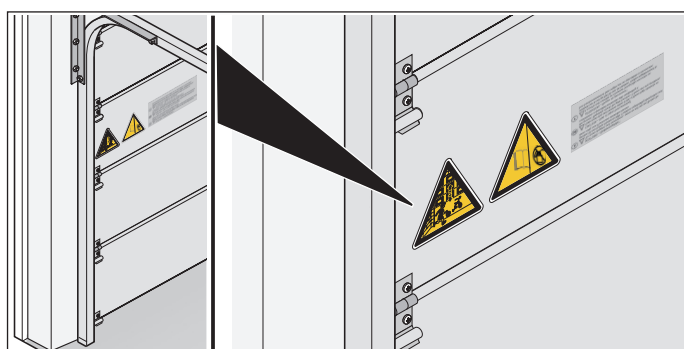
Fig. 1.2 Attach sticker to door panel
