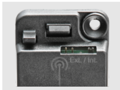
Connection for an external antenna.
