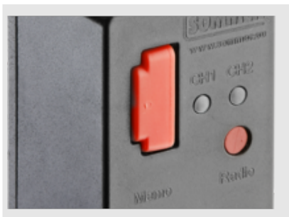
Slot with forced guidance for the Memo memory extension.
